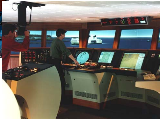
Fig. 8: Test setup for new Conning / ECDIS Display on Bridge 1 in Shiphhandling Simulator
