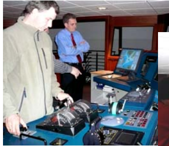
Fig. 8: Test setup for new Conning / ECDIS Display on Bridge 1 in Shiphhandling Simulator
